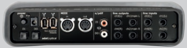
ADAT and TOS Link In/Out Power Input FireWire connections MIDI In/Out Digital S/PDIF Monitor/Line Outputs Line Inputs
